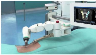
Mazor X Stealth robot-assisted spinal surgery system. Source: Medtronic
