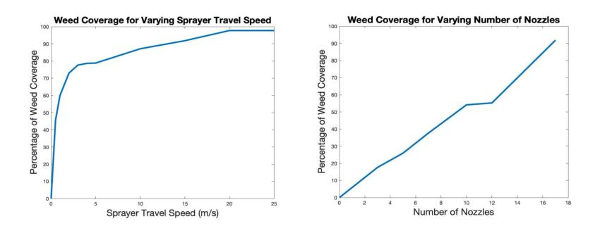
Fig. 4. Performance of Actuated Precision Sprayer (left) Vs Multiple Nozzle Sprayer (right).
