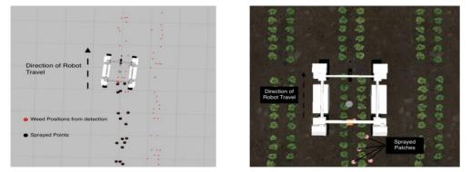
Fig. 3. Simulation of Actuated Precision Spraying in RViz (left) and Gazebo (right).
