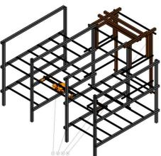
This will build up a timeseries dataset of growth conditions and images. The system comprises a mobile robot (1), shelves (2), elevator (3) and carriages (4).
